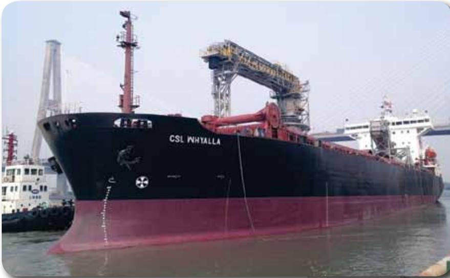
THE CSL WHYALLA IS USED FOR ACCESS TO SHALLOW PORTS INSTEAD OF BARGES WHICH REQUIRE TUGS.
